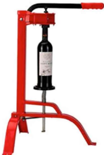
After each bottle is filled, cork it! Lift the corker plunger completely, put a cork into the cork chamber, stand the bottle on the base and hold the corker vertically on the neck of the bottle.
